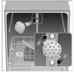
To ensure that the spray jet can reach all parts, arrange the baking sheets as illustrated
